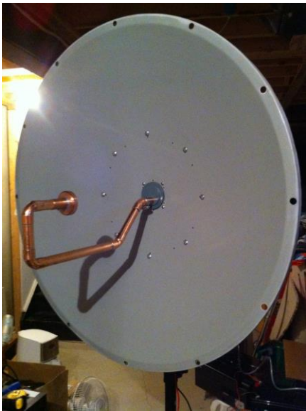
Parabolic Dish – Good gain to size ratio above 2 GHz. Commonly used for 5.8, 10, and 24 GHz
