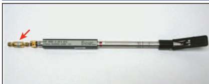
▲ Fig. 4 The adapter/sliding load configuration (LPC grade 3.5 mm socket adapter indicated by red arrow).
