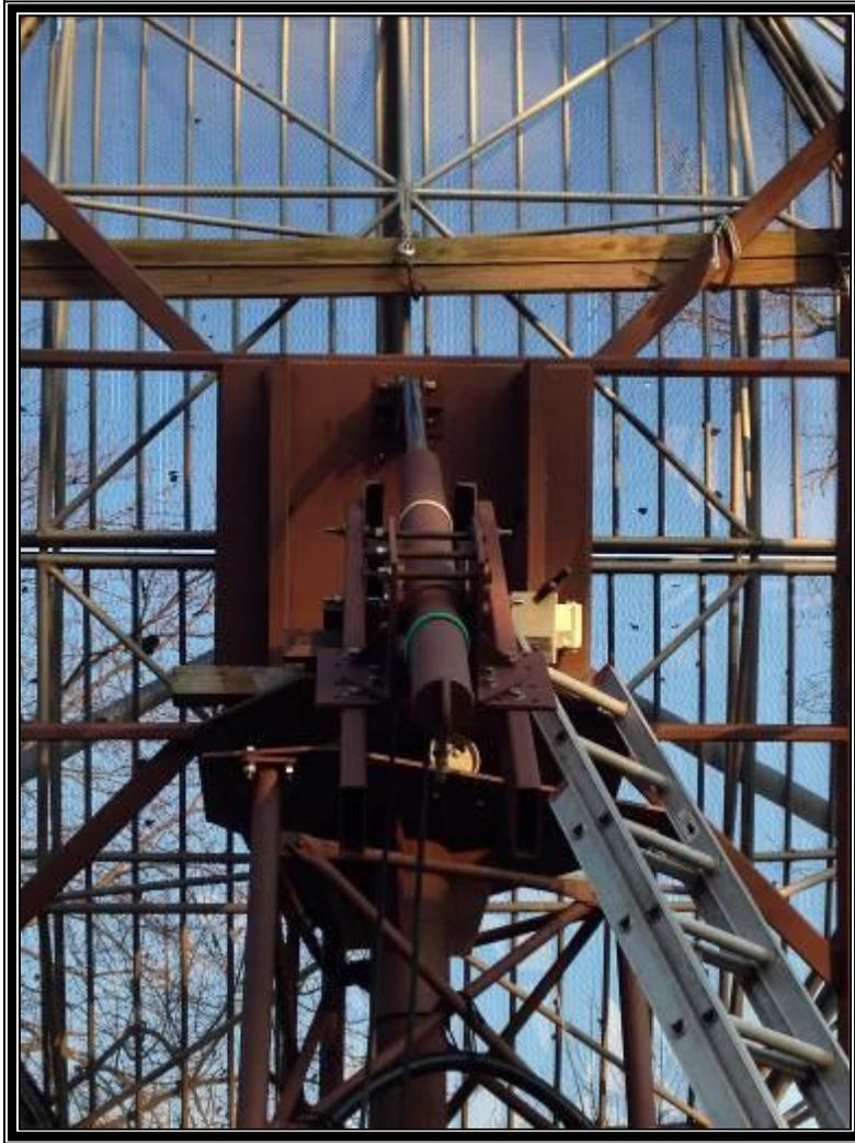
The new cylinder has significantly more volume for the working fluid, and consequently requires a larger reservoir volume. This has more or less topped out the available return side container, so an upgrade is going to be needed for the future. For now there is enough in it to exercise the cylinder, but it needs some headroom. The new reservoir will have to wait for temperatures to get a little warmer.
