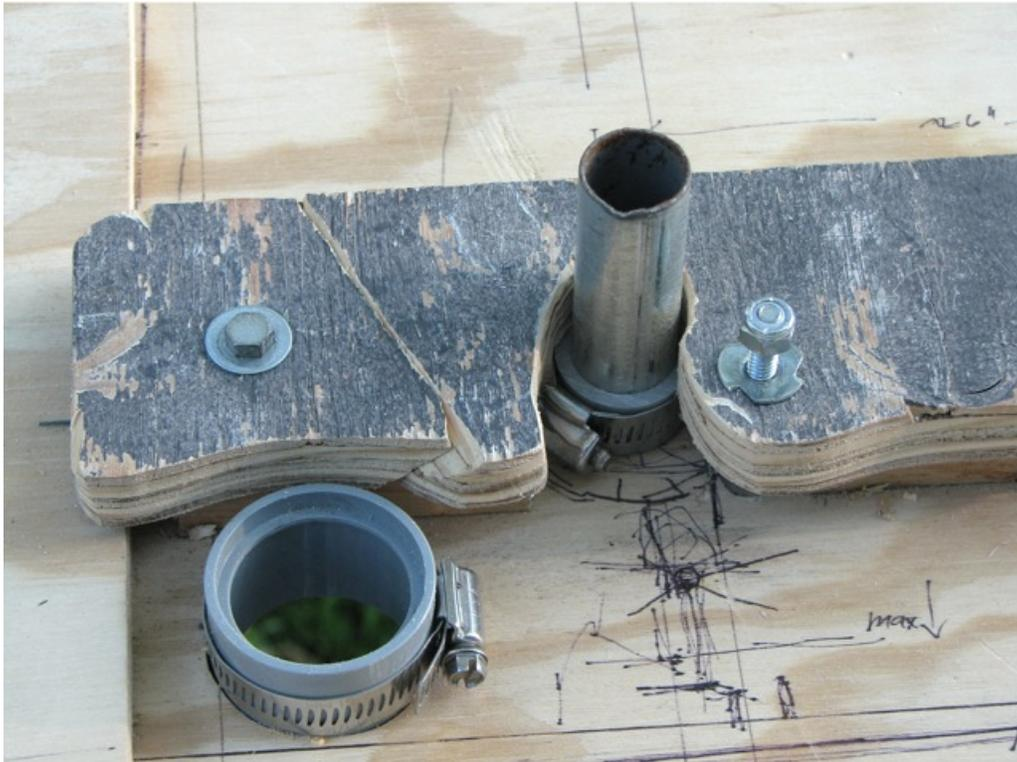
Gate detail--note bevel cut and coax port. Pivot bolt passes through deck.
