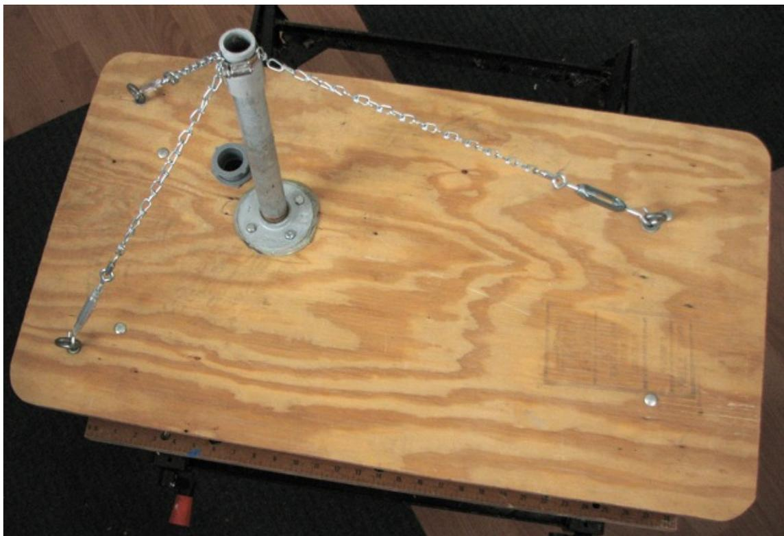
Tripod chain with 1" pipe and floor flange, note coax port.
