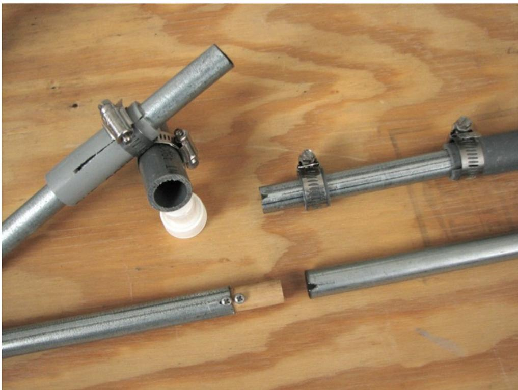
Detail: Collet and crossed clamp, stop and extension PVC, notched 5/8" and dowel pin.
