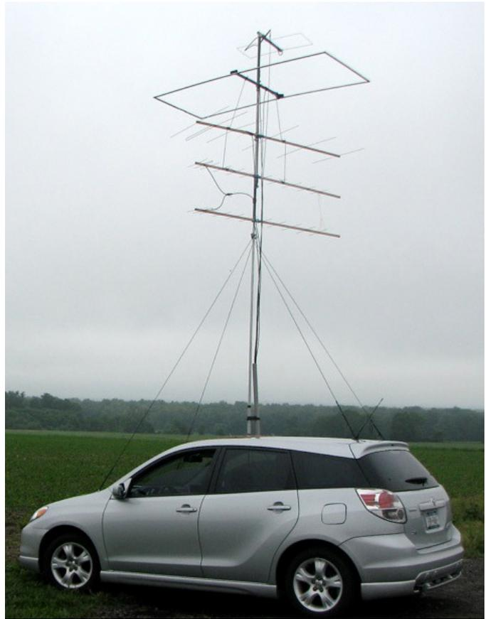
**Left:** Mast down, 2M Moxon above 6M Moxon, 2M Yagi, and stacked 432. **Right** Mast up, guys tight, antennas spread, top about 16 ft without additional mast extension.
