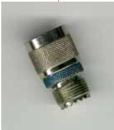
UHF Connector Faults . There are two major faults I can find with a UHF connector when it is being used on 432 and below: (1) the lack of weather proofing; (2) the lack of outer conductor finger contactors. With a proper tape wrapping job, I believe the weather proofing can be accommodated. However, the user must be sure that the internal "teeth" are properly seated,
